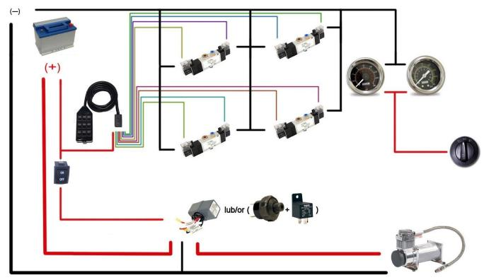
CAUTION! To connect the compressor, use at least 6 mm<sup>2</sup> diameter wire and a fuse 30-40A To connect the remote control and pressure switch, use a 0.25-0.5 mm square diameter wire and a fuse around 7.5A
