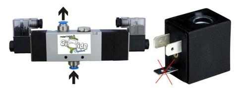
CAUTION! Only connect the control wires of the 2 parallel pins to the coil, the 3rd pin should stay disconnected!
